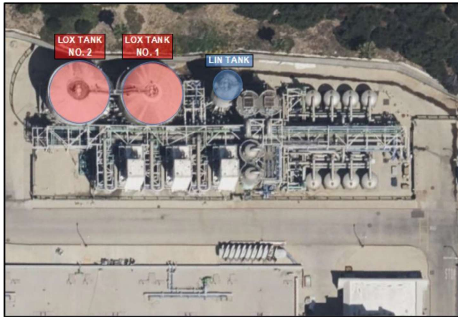
Figure No. 1: LOX and LIN Tanks at HWRP Cryogenic Facility
